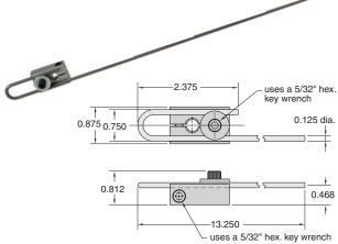
**Arm:** Steel 1/8" rod 13" long retained by screw clamp; the rod may be shortened and/or bent to desired shape
